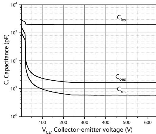
**Figure 4. Typical capacitance**
